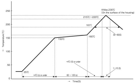
$Temperature\ measurement\ psrt: Terminal\ lead\ part.\ But\ the\ temperature\ on\ the\ surface\ of\ housing\ is\ 230^{\circ}C (max.)$
