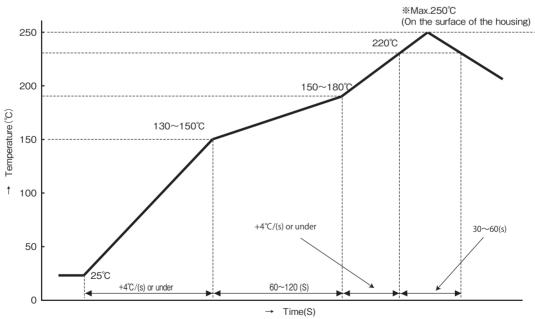
$Temperature\ measurment\ part: Terminal\ lead\ part.\ But\ the\ temperature\ on\ the\ surface\ of\ husing\ is\ 250\% (max.)$
